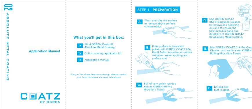
Use OSREN COATZ 01A Pre-Coating Cleaner to remove any polishing oils and to ensure the best possible bond and durability of OSREN COATZ 02 Absolute Metal Coating. Mist OSREN COATZ 01A Pre-Coating
